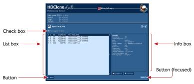
fig. 7: Graphical control elements (1)
